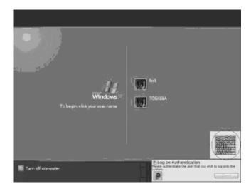
3. In the Windows Log-ON window, scan the fingerprint of your right index finger. Make sure that scanned fingerprint is displayed on the frame of [Logon Authentication] in green and you can log on.
