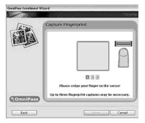
6. After displaying [Verify Fingerprint], scan the fingerprint of your right index finger on the finger sensor again. The message of "Verification Successful" is displayed. Click [Next] button.
